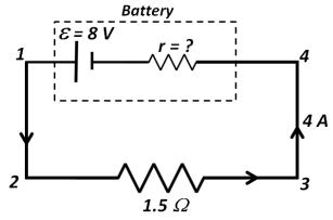
11. What is the potential difference measured across the light bulb terminals between points 2 to 3?(A) 1.5V(B) 2V(C) 6V(D) 8V
