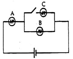
7. Given three identical light bulbs connected with a switch and ideal emf as shown.
