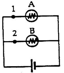
6. The figure above represents two identical light bulbs, A and B, that are connected to an ideal emf. Then, a very low resistance wire is attached joining points 1 and 2. As a result, \_\_\_\_\_.
