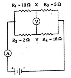
19. Given four resistors joined in two parallel branches as shown. The voltmeter, V, reads 8.5 volts with point Y the plus or higher end. The current in the 2 ohm resistor is \_\_\_\_\_ A.
