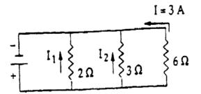
3. Given three resistors, (2 ohms, 3 ohms, and 6 ohms, arranged in parallel with an ideal emf. The directions of the currents in the resistors are shown. The current is 3 amperes in the 6 ohm resistor.
