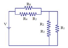
12. How does the total current and effective resistance of the circuit change, it at all, if the battery used in #11 remains the same, but you insert one more resistor of unknown non-zero magnitude in parallel with  $R_1$ ?
